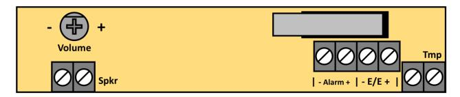
The  $16\Omega$  speaker in this unit is pre-wired to the speaker terminals of the PCB.
